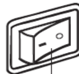
Power/light switch "OFF"
