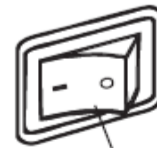
Power/light switch "ON"
