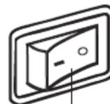
Power/light switch "OFF"
